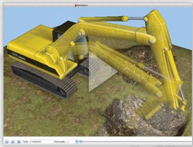
Vary the length of the cylinder controlling the boom at different time points and immediately see the resulting movement
