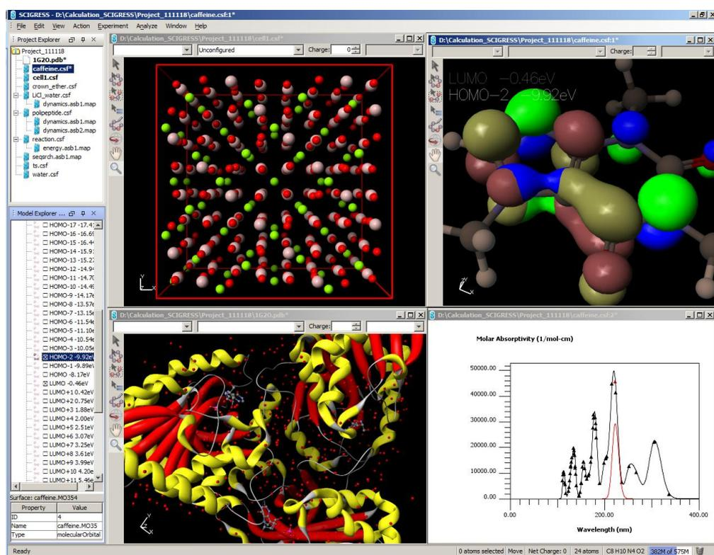
Molecular mechanics calculations can be performed on organic and inorganic molecules containing all elements of the periodic table using variety of force fields. Force field parameters can be modified by the user. SCIGRESS includes CONFLEX for automated global minimum searching and systematic generation of low-energy conformers for molecules of any shape, including ring systems.
